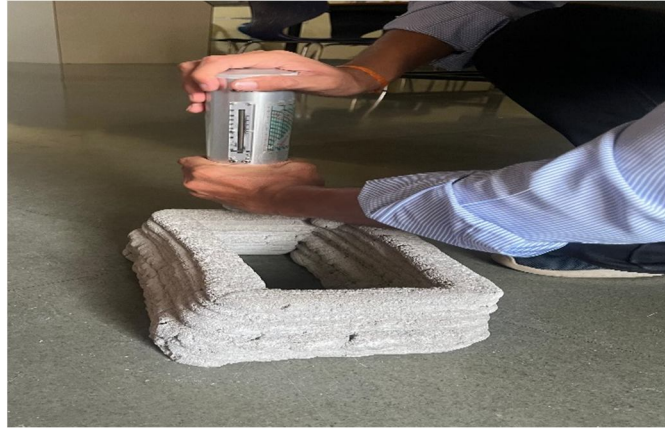
Fig Rebound Hammer test perpendicular to the layers
