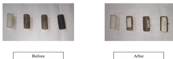
Figure 7. compression tested samples before after
