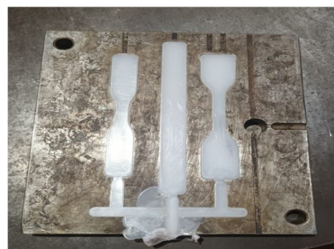
Figure 7. HDPE injection molding specimen in die
