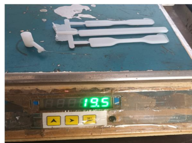
Figure 6. HDPE after injection molding specimen weight
