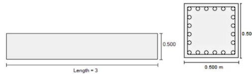
Figure 6: Design of Column ( 1-4 floor)
