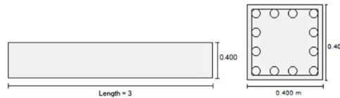
Figure 7: Design of Column ( 5-8 floor)
