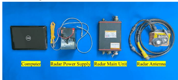
(a) RIS Series Ground Penetrating Radar
