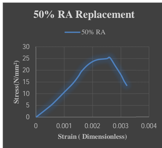
Graph 9: Stress-Strain Curve for 50% Recycled Aggregate
