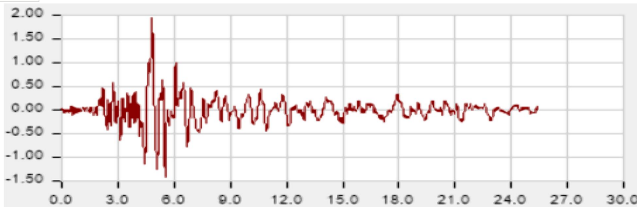
Acceleration vs Time data along Horizontal N-W Direction
