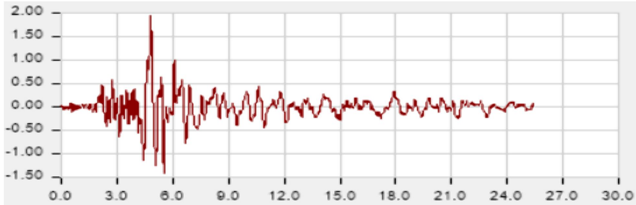
Acceleration vs Time data along Horizontal N-W Direction
