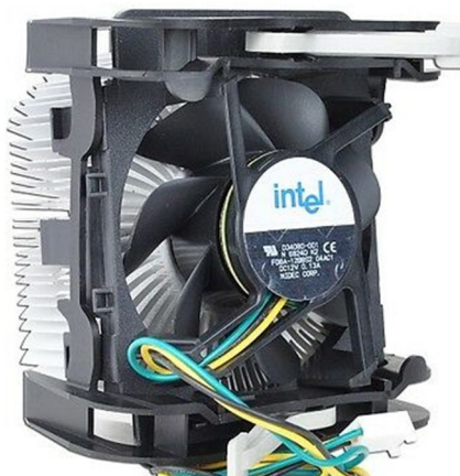
Fig. Exhaust fan with Aluminum heat sink
