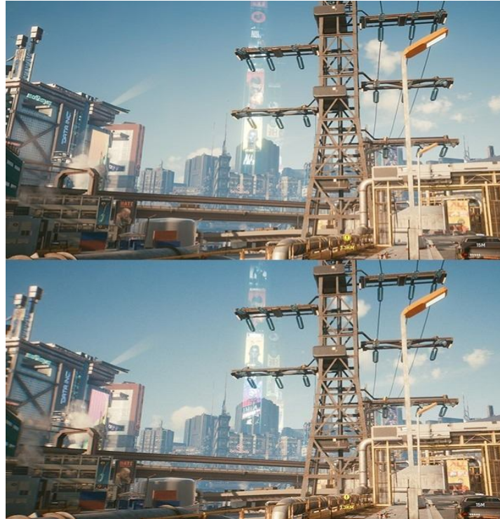
Fig. 1.5 Ambient Occlusion and Dispersion with and with-out Ray Tracing Implementation
