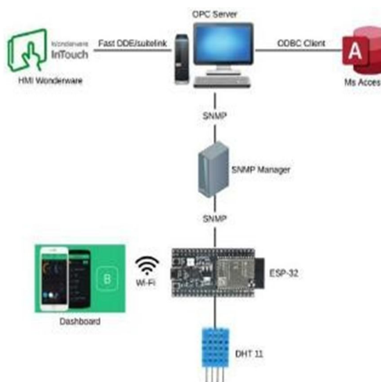
Figure 3 System architecture of IoT
