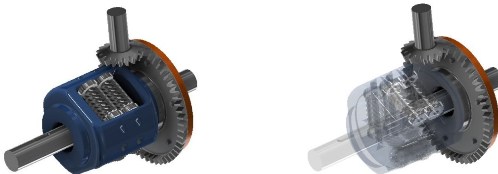
Fig. 1 A geometrical model of the Torsen differential
