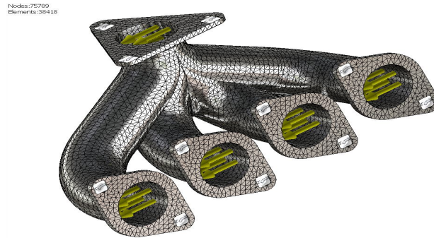
Fig. 4 Exhaust gallery meshing
