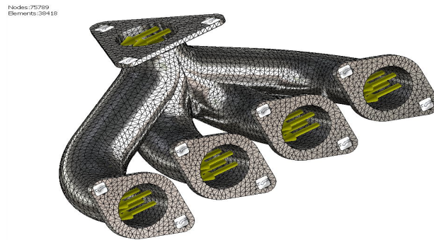
Fig. 4 Exhaust gallery meshing
