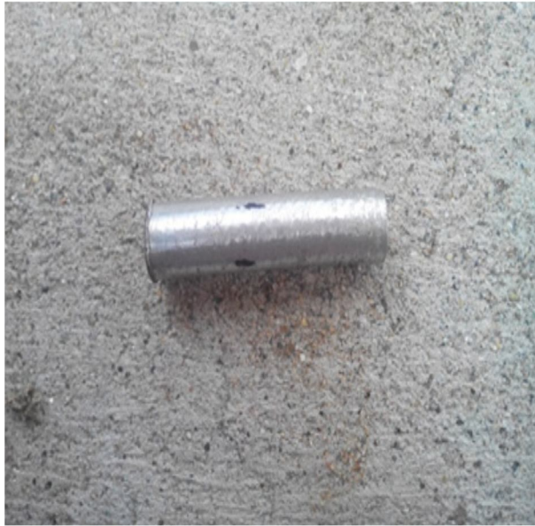
Fig. 3.7 Wear test specimen
