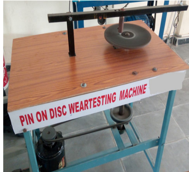
Fig3.8 Pinon disc wear testing equipment
