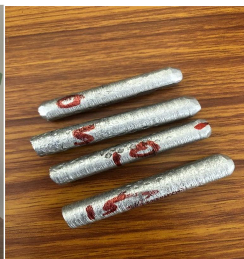
Fig. 3.6 Hardness test specimens
