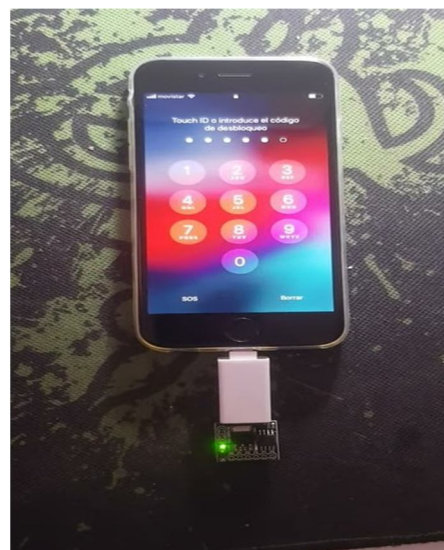
Fig.7.Connecting ATtiny 85 to mobile
