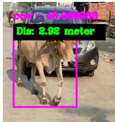
Fig. 8: Accurate animal detection and Distance Estimation
