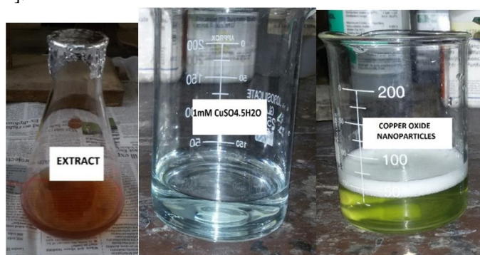
Figure 1. Colour change of copper sulphate solution before and after synthesis of nanoparticles
