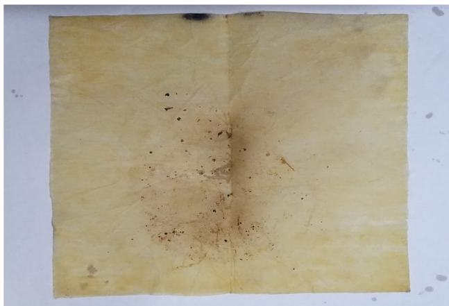
Figure 22: Non coated polypropylene filtration membrane at the end of 4 th day of machining process
