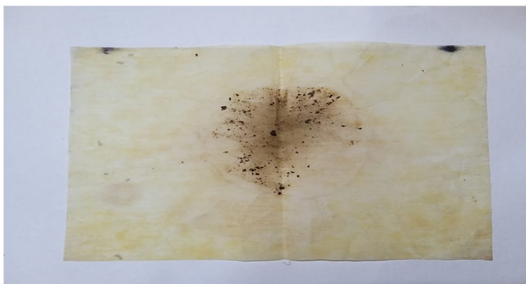
Figure 23: Coated polypropylene filtration membrane at the end of 4 th day of machining process
