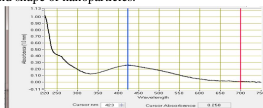
Fig. 2: UV-Visible absorption spectra of synthesized silver nanoparticles
