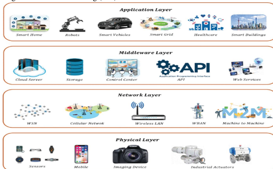
Figure 3: Industrial IoT system architecture [41].
