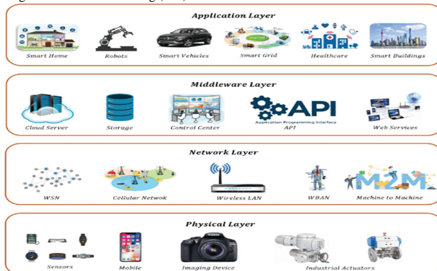
Figure 3: Industrial IoT system architecture [41].
