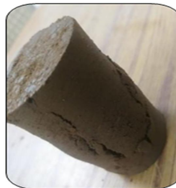
UCS SAMPLE FAILURE PATTERN
