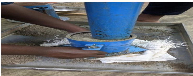
Modified proctor test (Heavy compaction)
