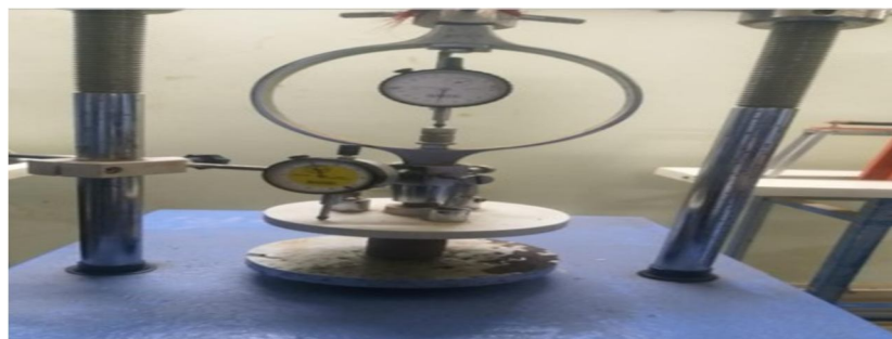
UCS Testing machine set up
