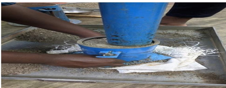
Modified proctor test (Heavy compaction)
