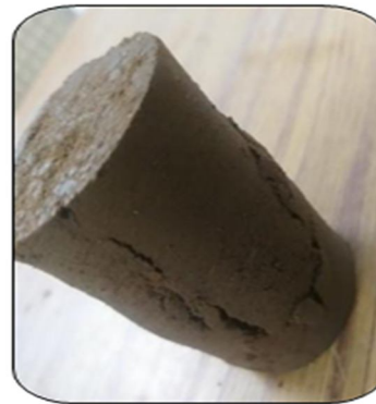
UCS SAMPLE FAILURE PATTERN
