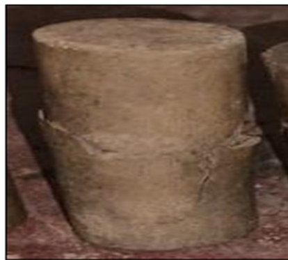
UCS SAMPLE FAILURE PATTERN
