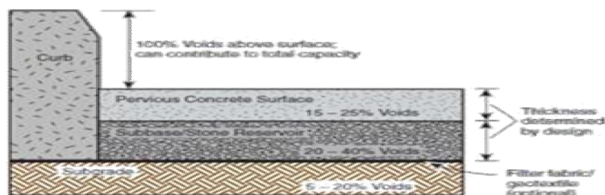
Fig 9 Typical cross section of pervious concrete Pavement
