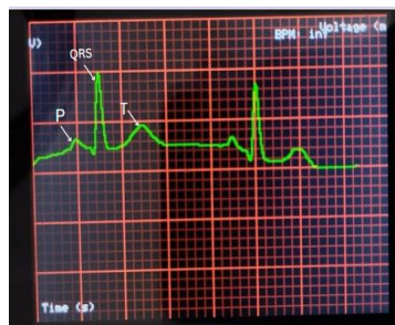
Fig. 11b PQRST Waveform Captured During Testing
