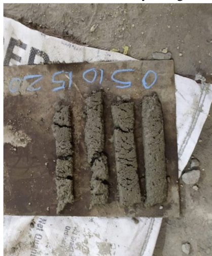
Figure 3: Open time test done for time interval of 5 min.
