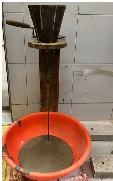
Figure 5: Marsh cone test assembly
