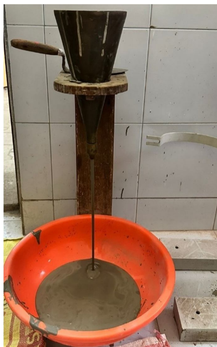
Figure 5: Marsh cone test assembly
