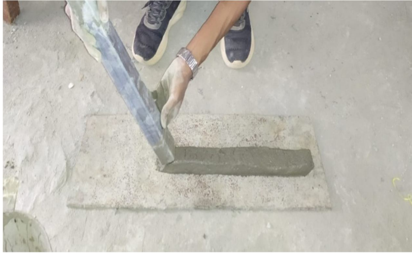
Figure 2: Prototype (GI pipe) used for extrudability testing
