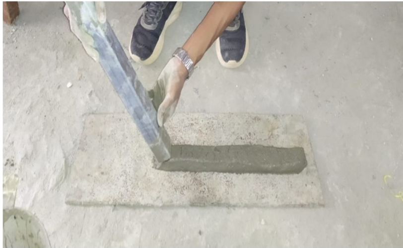
Figure 2: Prototype (GI pipe) used for extrudability testing
