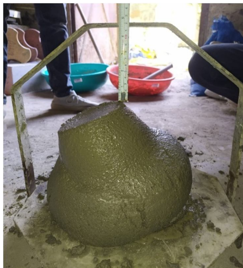
Figure 6: Pumpability was evaluated using an ASTM C143-compliant standard slump cone
