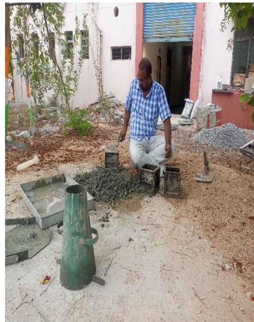
Fig. 4 Concrete Cube casting
