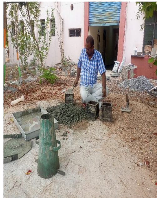
Fig. 4 Concrete Cube casting
