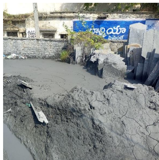
Fig. 2 Cuddapah Slab Polishing Waste
