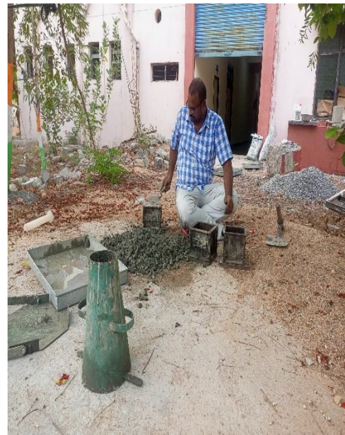
Fig. 4 Concrete Cube casting
