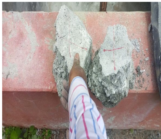
Fig.6 Sample failed during Curing (50% replacement of cement with Barytes)
