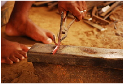
Fig.7 Bending Metal to Form a Shape
