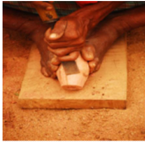
Fig.14: Shaping Wood Using Chisel
