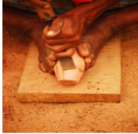
Fig.14: Shaping Wood Using Chisel
