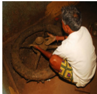
Fig.11: Moulding Clay on Potter's Lathe
