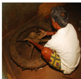
Fig.11: Moulding Clay on Potter's Lathe
