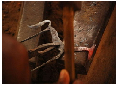
Fig.8: Hammering to Give a Finished Look
