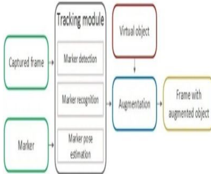
Fig. 3 Working Model of AR core
