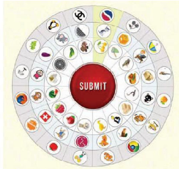
Figure 7. Three chosen photographs are lined together in a certain way. The user will click the submit button after aligning [1].
