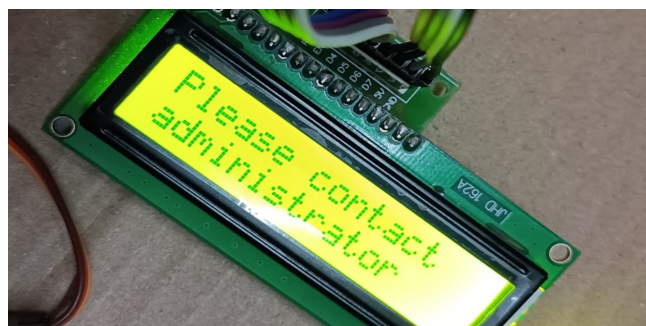
Fig. 16. LCD Output When an Unauthorized Vehicle Enters
