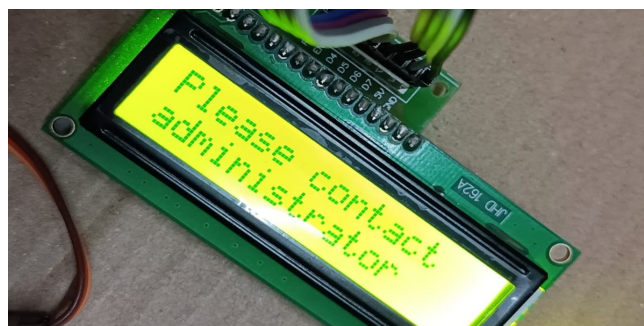
Fig. 16. LCD Output When an Unauthorized Vehicle Enters
