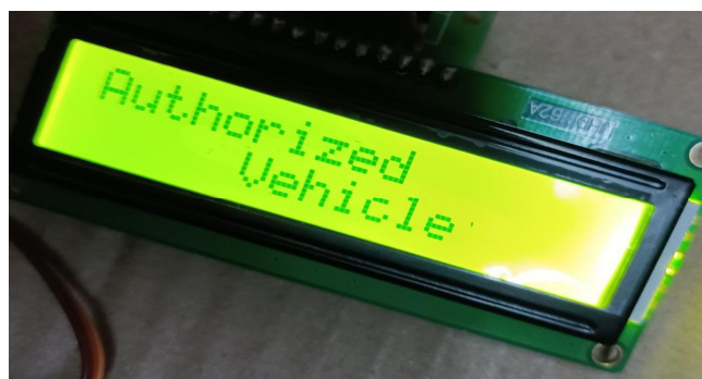
Fig. 13. LCD Output When an Authorized Vehicle Enters
