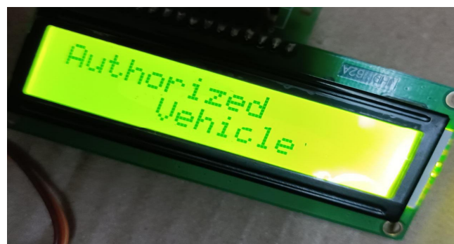
Fig. 13. LCD Output When an Authorized Vehicle Enters
