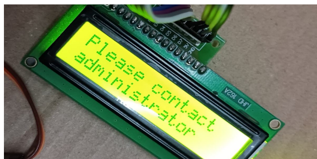
Fig. 16. LCD Output When an Unauthorized Vehicle Enters
