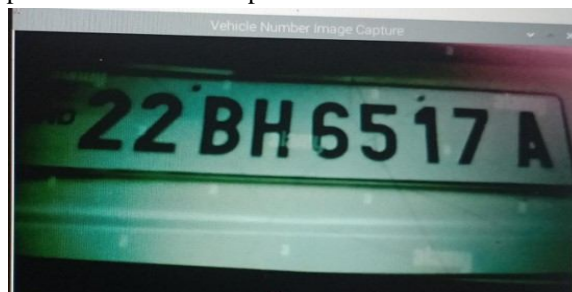
Fig. 3. Image Captured by Raspberry Pi Camera after IR Sensor detected a vehicle
