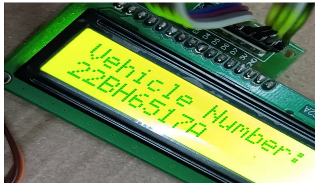
Fig. 11. LCD Output After Extracting Vehicle Number from the Captured Image
