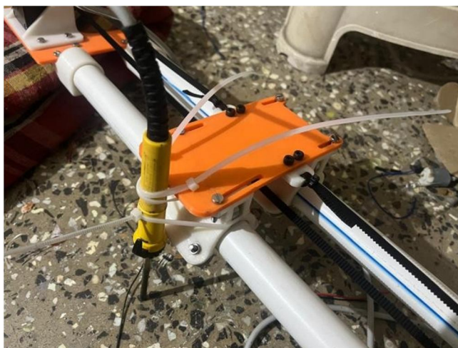
Fig4. display the soldering gun connected with the conveyor belt. stepper motor moves the soldering gun using conveyor belt
