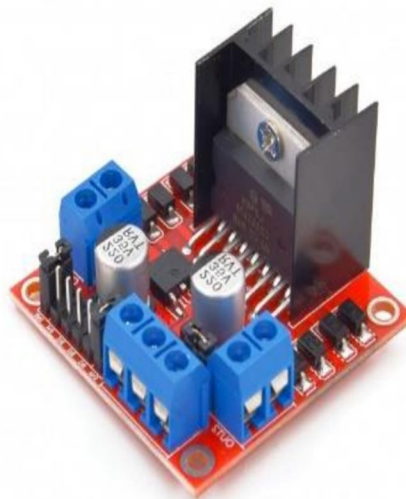
Figure 4 H-Bridge for Motor and Sensor power distribution
