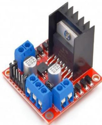
Figure 4 H-Bridge for Motor and Sensor power distribution
