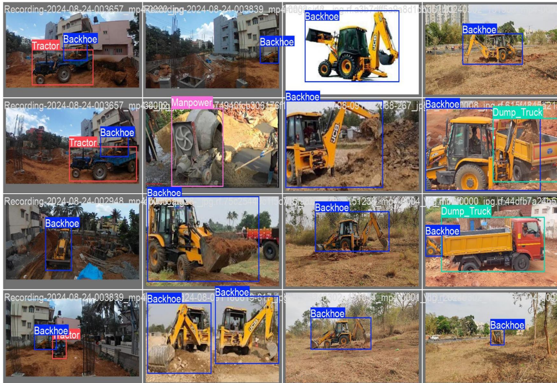
Fig 1: Object Detection in Construction Sites
