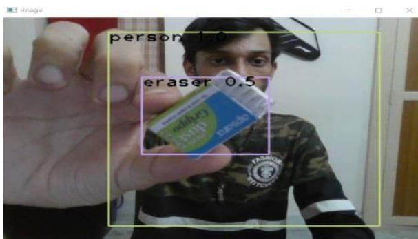
Fig. 3. Detection of Person and Eraser with Label and Confidence Value
