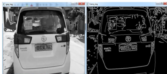
Fig. 2.a. Grayscale image of inputted vehicle & b. Canny image is generated by inputting Grayscale image
