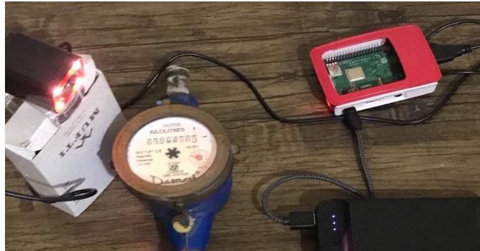
Fig. 5 Automated Water Meter Reading System
