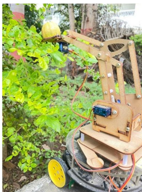
Figure 8: Robotic arm plucking lemon
