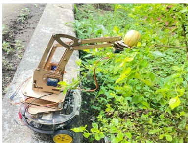
Figure 7: Robotic arm plucking lemon
