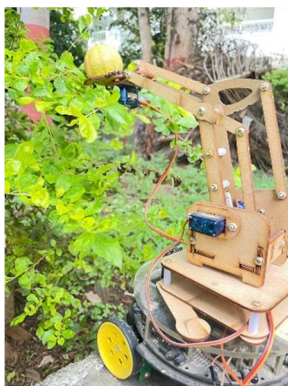
Figure 8: Robotic arm plucking lemon
