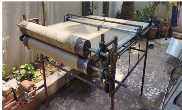
Fig.8. Main setup of automatic lamination cutting machine
