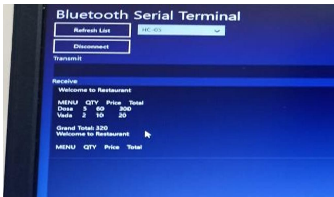
Figure 9. Bluetooth-received order displayed on computer
