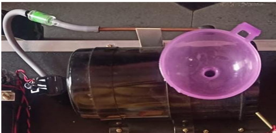
Fig 9. Pesticide Spraying Tank
