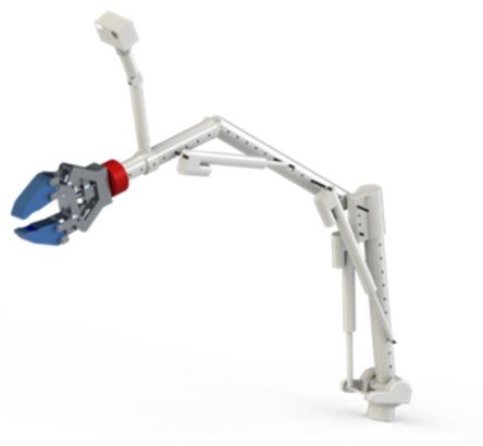
Fig 15. Robotic arm with the gripper and guiding camera
