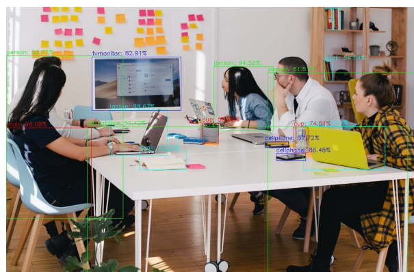
Figure 23: Detections in an image using YOLOv4
