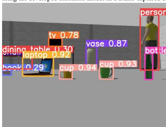
Figure 25: Detections in ROS environment using ensemble model
