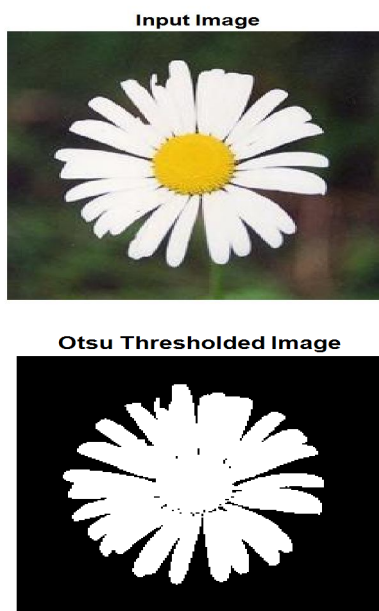
Figure 3: Input Image with Thresholded Output
