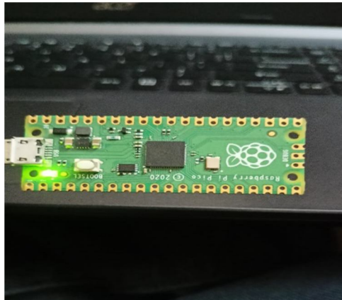
Fig.2.1 The raspberry pi pico connected to a system with the required code
