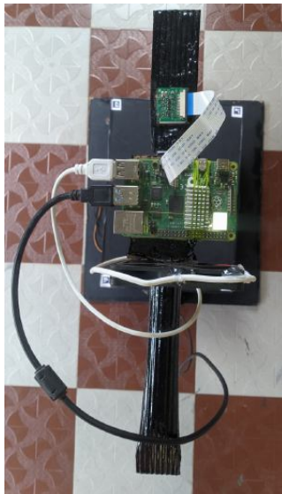
Fig.7 Raspberry Pi and PiCamera
