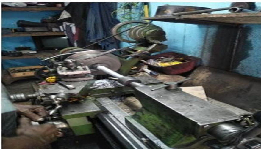
Fig: Turning process for Casting Component
