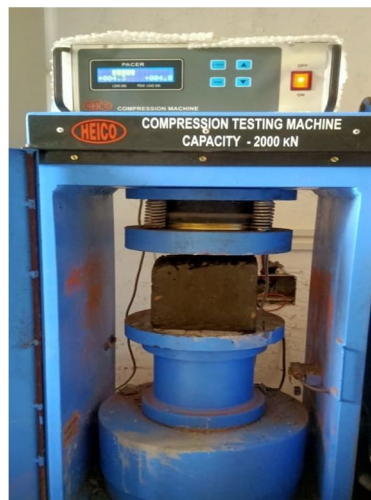
Figure 3.3.4: Concrete cube placed under Universal Testing Machine
