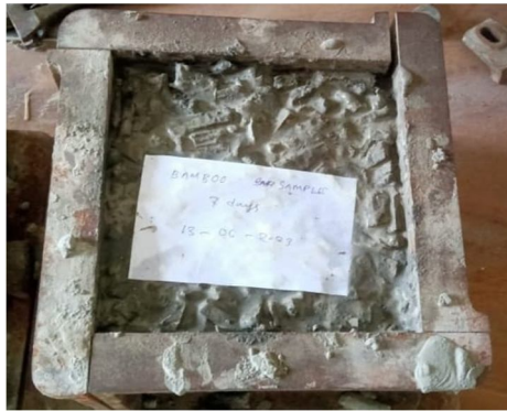
Figure 3.3.2: Natural dried cube of bamboo aggregate
