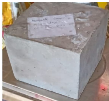
Figure 3.3.3: Natural dried cube of stone aggregate
