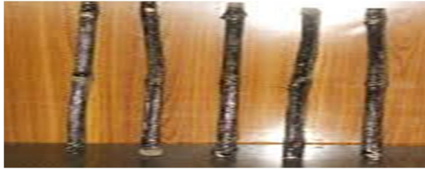
Figure.3.2: Bamboo sticks after treatment with coal tar.
