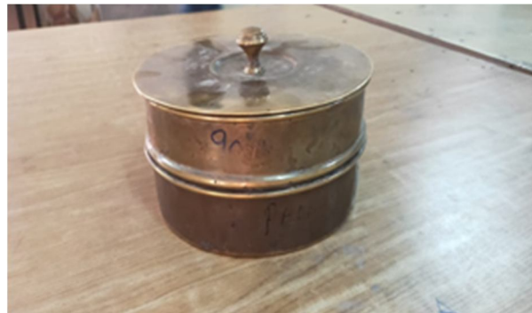
Fig. 4.3 Determination of fineness of cement by dry sieving.
