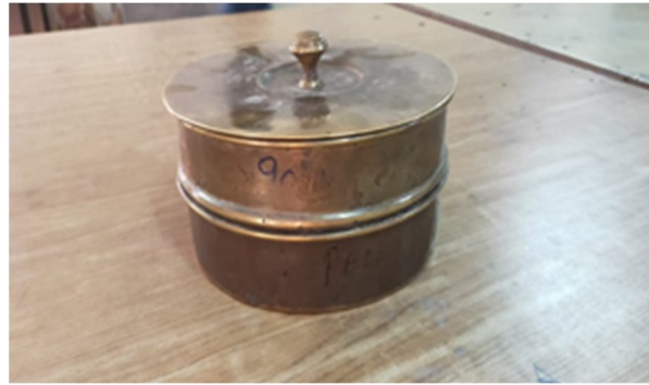
Fig. 4.3 Determination of fineness of cement by dry sieving.
