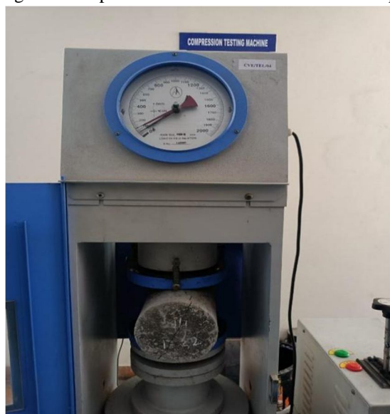
Fig. 4.7 Determining the split tensile strength of the cylinder's through CTM
