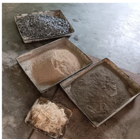
Fig.4.2 It shows materials (a) Fine aggregate (b) Coarse aggregate (c) Cement
