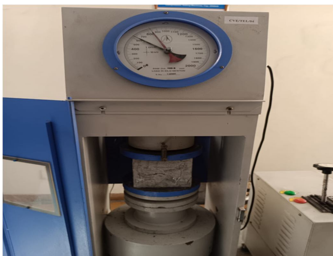
Fig.5.1 Determining the compressive strength of the cube through CTM for 28 days
