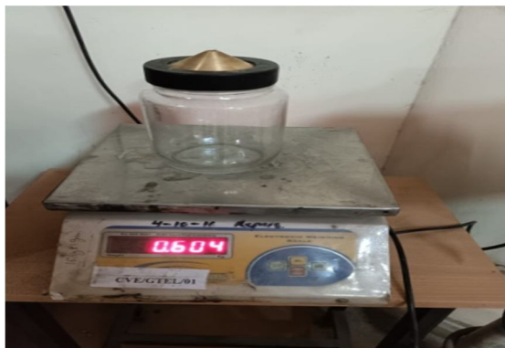
Fig. 4.5 Pycnometer being weighed
