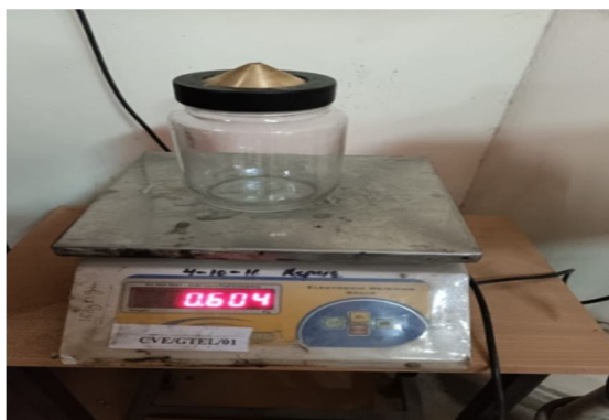
Fig. 4.5 Pycnometer being weighed
