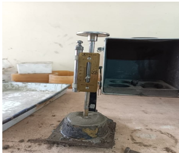
Fig. 4.4 Vicat Apparatus with Mould penetrates to a depth 5 to 7 mm from the bottom of the Vicat mould.
