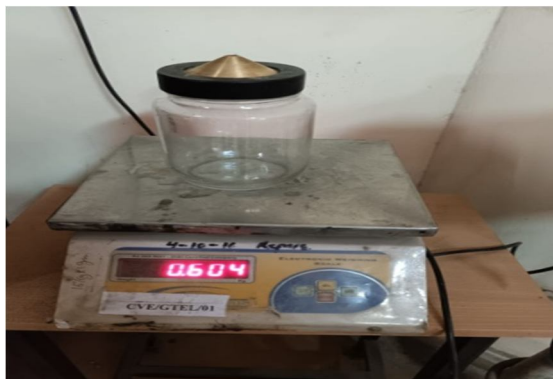
Fig. 4.5 Pycnometer being weighed
