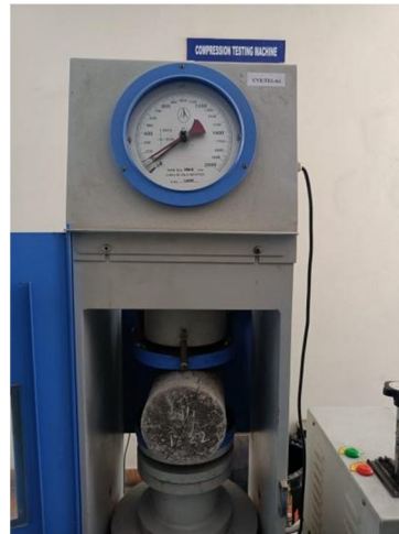
Fig.5.5 Determining the split tensile strength of the cylinder's through CTM for 7 days
