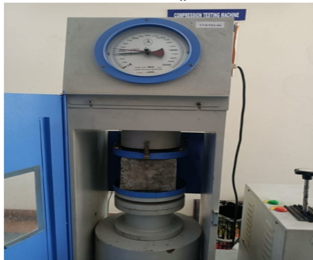
Fig. 4.6 Determining the compressive strength of the cube through CTM
