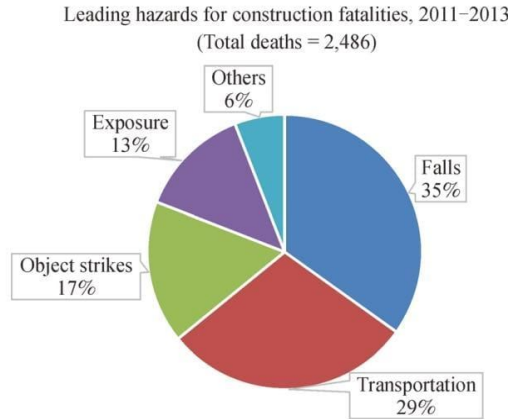
Fig. 2 Distribution of leading hazards that causes construction Fatalities.[2]
