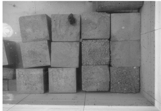
Fig.5.2.4 Curing of cubes
