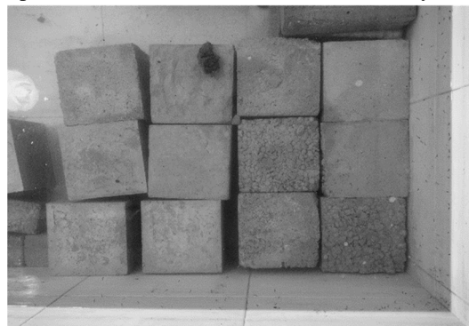
Fig.5.2.4 Curing of cubes
