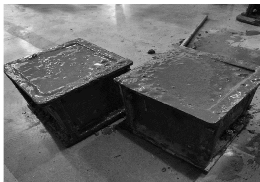
Fig.5.2.3 Casting of cubes
