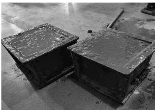
Fig.5.2.3 Casting of cubes
