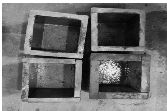
Fig.5.2.2.1 Preparation of moulds
