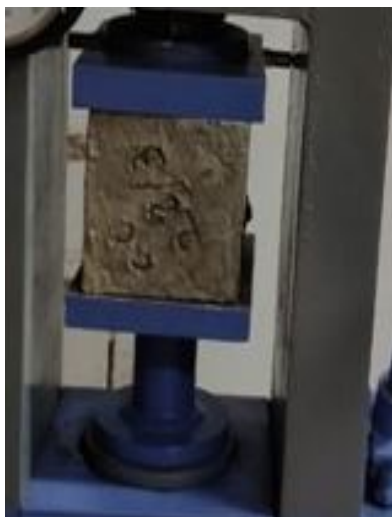
Fig. 10 Compressive Strength of Concrete Test
