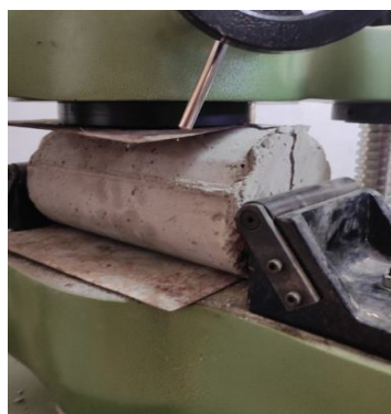
Fig. 12 Split Tensile Strength of Concrete Test
