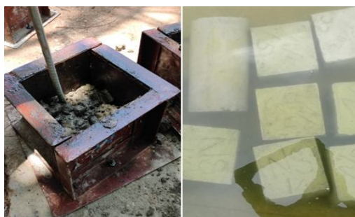
Fig. 7 compacting and curing of concrete
