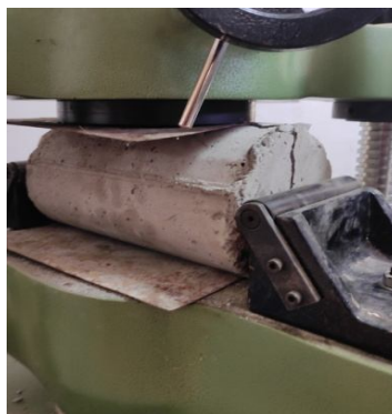
Fig. 12 Split Tensile Strength of Concrete Test
