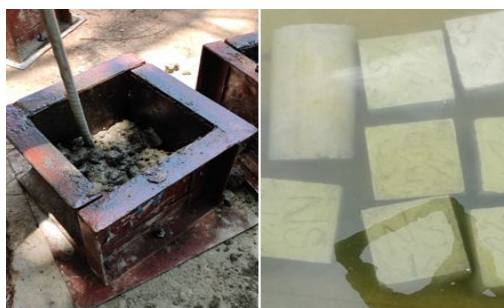
Fig. 7 compacting and curing of concrete
