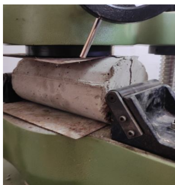
Fig. 12 Split Tensile Strength of Concrete Test
