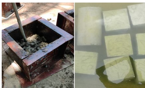
Fig. 7 compacting and curing of concrete
