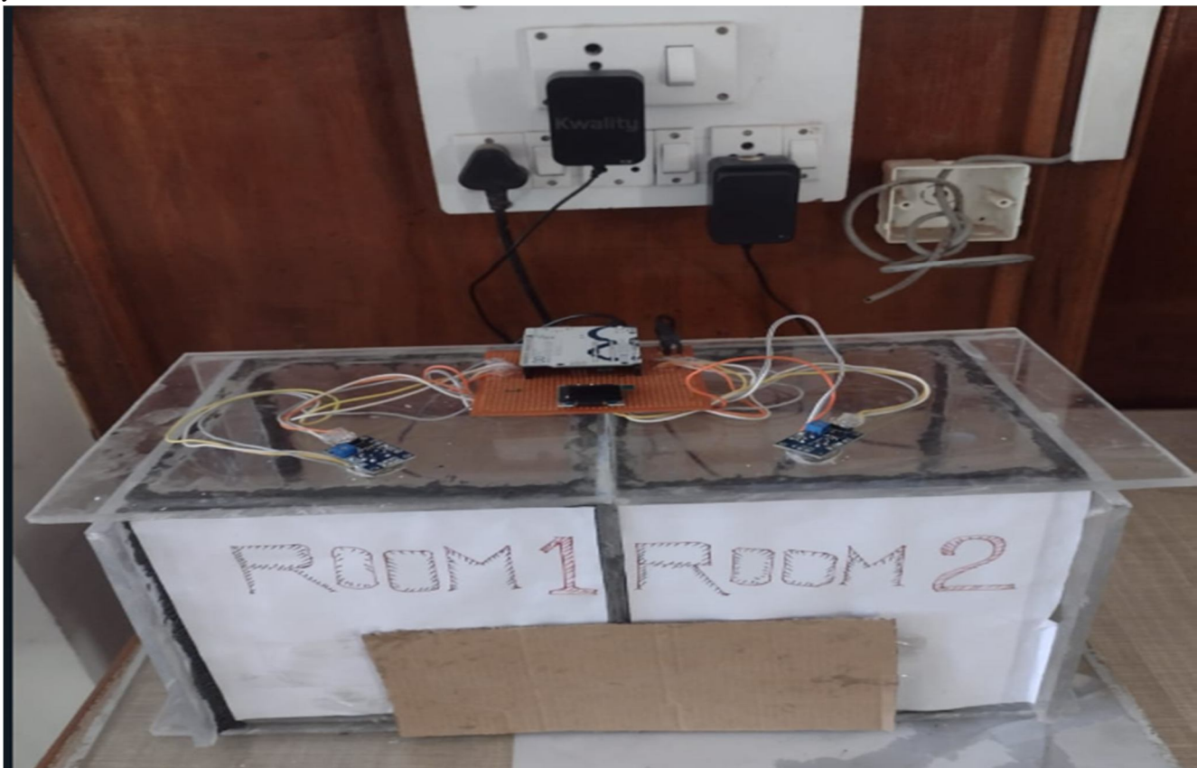
Fig.4 Carbon sequestration study chamber with MQ 135 sensors
