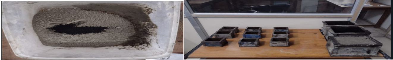
Fig.3 Mortar cubes and concrete cube preparation with walnut shell biochar enrichment.
