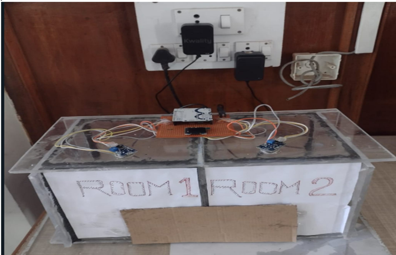
Fig.4 Carbon sequestration study chamber with MQ 135 sensors
