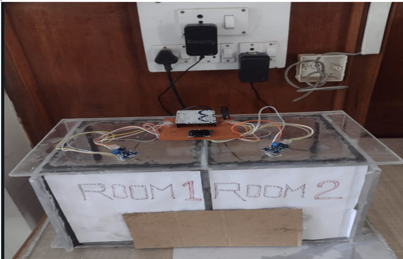
Fig.4 Carbon sequestration study chamber with MQ 135 sensors
